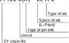
Plain chain consists of 'SY chain No" and "Type of pin link". Attachment chain has one space between "Type of pin link" and "Space of attachment".
